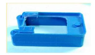
Cut the tender shell as shown and cut back the tool boxes to the edge of the hinges.
