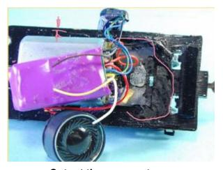
Cutout these areas to accommodate a 1/2" speaker and baffle and the capacitor. The cutout should go no wider than the lug at the arrow.
