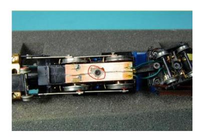
Cut a piece of PCB to cover the bottom of the loco. 1/16" is shown. That won't work, D-oh!!, the tender connector wires will short out on turnouts. I replaced it with 1/32" thick and that worked. If you can't find PCB that thin an alternate is brass shim stock glued to styrene like the strips on the tender. Relieve the board at the gear. Electrically separate the sides and remove the copper clad from around the screw.
