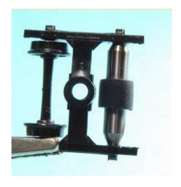
Keep taking material out of the sides until the sideframe sides are flat.
