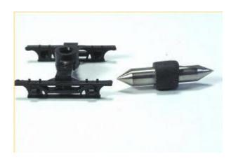
A "Reboxx HO T-100 Exxact Socket Tool" is used to open up the sideframes to accept the longer axles.
