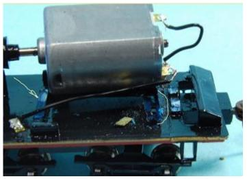
Remove the front motor mount and relieve the frame at the back of the motor well so the motor "snaps" in.
