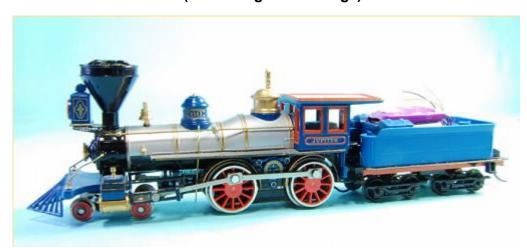
This is our "beta" locomotive, excuse the disrupted cross heads and other cosmetic problems. The loco has a "daylighted" cab, Soundtraxx Tsunami sound, prototypical spacing between loco-tender, bigger tender wheels and will crawl along.
