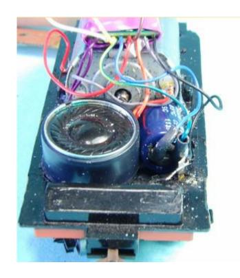
I am using a Soundtraxx Micro Tsunami C-16 version, it has more old locomotive sounds. The speaker is a Soundtraxx 1/2" using their baffle.
