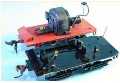
The newer tender frames have a recess for the motors while the older pancake motor frames don't and the electrical pickups are different. The old ones will require more mods but will work.
