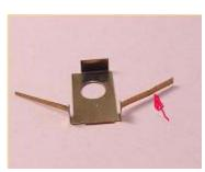
Spread the "wings of a Kadee #5 Centering spring and straigten out the bend wing.
