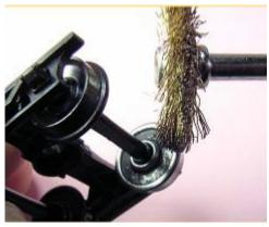
The Kadee wheelsets have a coating that doesn't conduct electricity. Put the wheelset in an EXPENDABLE truck frame and burnish the wheels with a brass brush in a motor tool.
