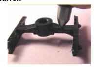
Use the truck reamer to break the edge of the tapped hole to make the insertion of the screw easier.
