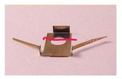
The spring should be symmetrical after tapering. Cut off the back portion of the spring.
