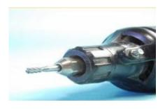
A motor tool with a 1/8" diameter burr makes the conversion easier. I find this the most controllable size.
