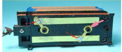
Remove everything not shown from the bottom of the tender frame. Slide 3/16" wide x .002 thick brass strips under the tender contacts so the truck wipers touch the strip. Solder them as shown and ACC the strips to the frame when the solder has cooled.
