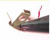
Taper the straight wing by holding the wing with pliers.
