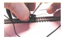
Test the electrical pickup with an automotive tester while rolling the truck along the track. Test one wheel at a time. Ajust the wiper for least rolling resistance.
