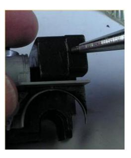
Mark the cab to confrom to the boiler and to the end of the frame.
